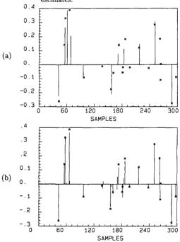
Deconvolved results associated with  $v_2(k)$  and (a) Figure 3 SNR=10, (b) SNR=10000, respectively. \*'s denote true spikes and bars denote estimates.
